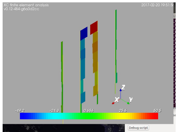
Figure 54: ELUmaxMz: maximum internal moment M_z . Inner columns, internal shear force in local direction z [kN]
